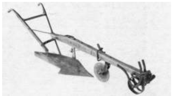
Fig.10 – A walking plough. Note the front resting on a small wheel. At the rear is the handle with which the ploughman guided the plough. The plough was hitched to a team of oxen or horses. (See Fig.13)
