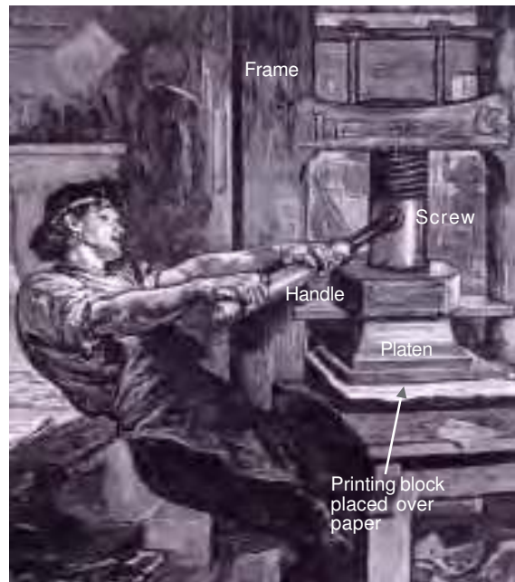
Fig. 6 – Gutenberg Printing Press. Notice the long handle attached to the screw. This handle was used to turn the screw and press down the platen over the printing block that was placed on top of a sheet of damp paper. Gutenberg developed metal types for each of the 26 characters of the Roman alphabet and devised a way of moving them around so as to compose different words of the text. This came to be known as the moveable type printing machine, and it remained the basic print technology over the next 300 years. Books could now be produced much faster than was possible when each print block was prepared by carving a piece of wood by hand. The Gutenberg press could print 250 sheets on one side per hour.
