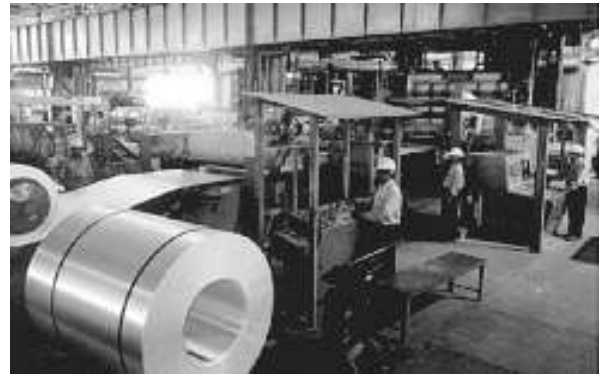
Fig. 6.6: Strip coating mill at smelter of NALCO
